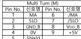
<Encoder Connector 핀 배열>
